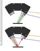
IN0 = HIGH backward reflection line scan detector position lightning source for backward reflection IN0 = LOW forward reflection line scan detector position lightning source for forward reflection
