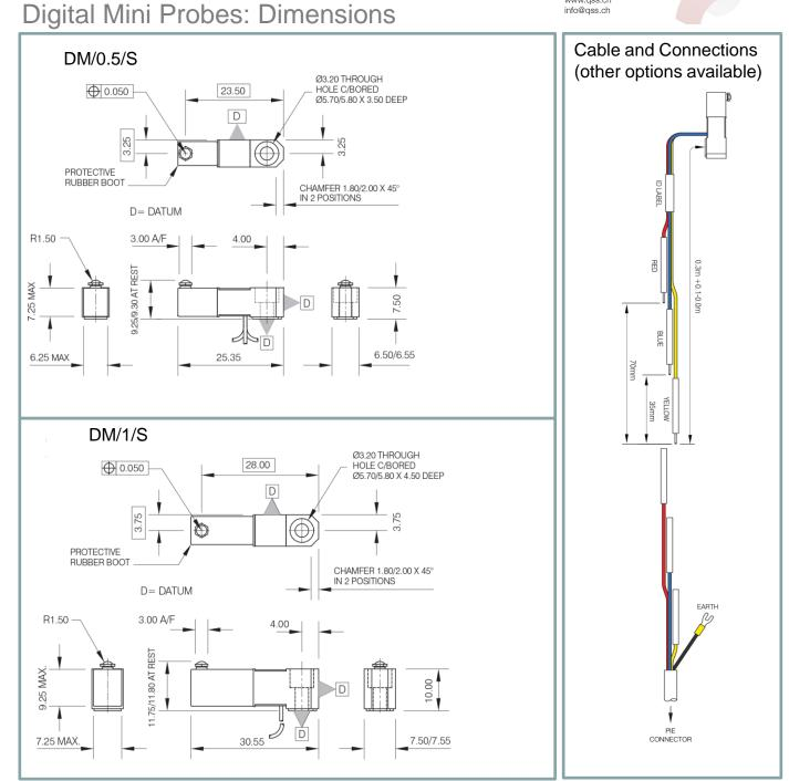
All dimensions are nominal only for accurate drawings download the correct Sales Application Drawing from the Solartron Metrology Website
