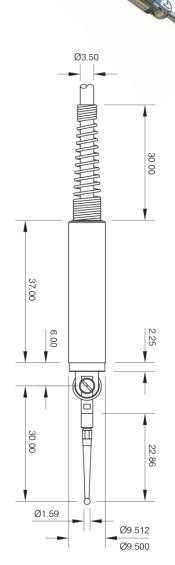
All dimensions are nominal only for accurate drawings download the correct Sales Application Drawing from the Solartron Metrology Website
