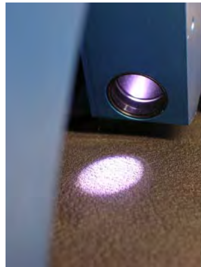
Examination of leather surfaces with respect to their gloss behavior
