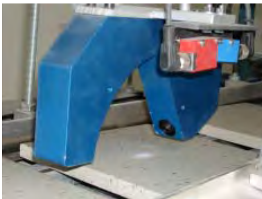
Gloss degree monitoring at plates of stone
