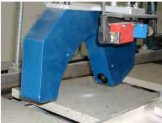
Gloss degree monitoring at plates of stone
